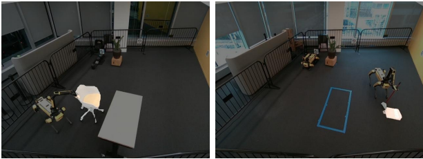
Fig. 5: Grounded SAM/Detic Visualization: We run open-vocabulary text-based detection to obtain bounding boxes, followed by a segmentation model to obtain an object mask, visualized for chair (left) and sweeping (right). This can be used along with depth observation from calibrated cameras in the environment (including the robot’s egocentric vision sensors) to obtain 3D object point cloud.
