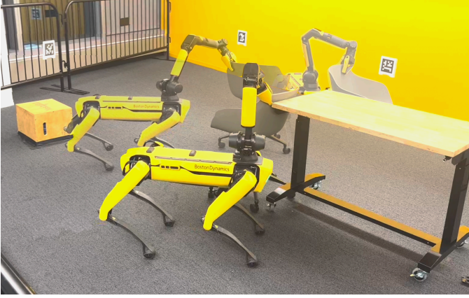
Fig. 8: Left: The prior (RRT* with incomplete model) gets stuck in a collision with the table and is unable to recover as the planner does not have a model of chair-table interaction dynamics. Right: Our approach effectively recovers from collisions to complete the task.
